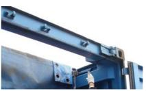
2. Removable Rear Top Rail For large machinery or bulk items that need to be slid in through the container doors, the rear top rail can be removed necessitating access.
