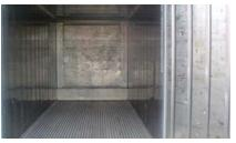
1. Aluminium 'T-Section' floor These containers have a standard Aluminium 'T-Section' Floor.
