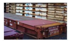
3. Flush Folding Makes for loading over-length items onto a base while still allowing for ease of handling.
